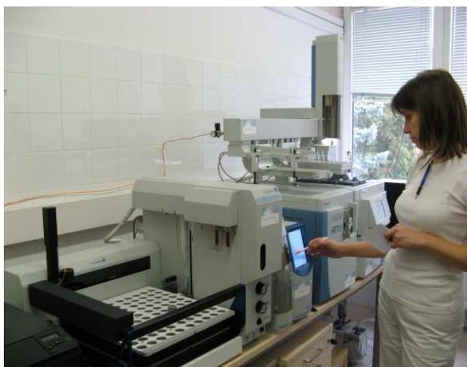
**Gas chromatography mass spectrometer (GC-MS):** The equipment is able to measure organic micro-pollutants. This equipment allows components to be measured reliably with high sensitivity in the expected measurement range.
