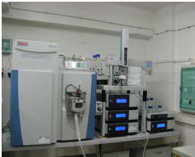
**HPLC-MS equipment:** The equipment is suitable for defining organic components that the Environment Protection Measurement Centre was not able to test before. These components are for example pharmaceutical residues, i.e. diclofenac.
