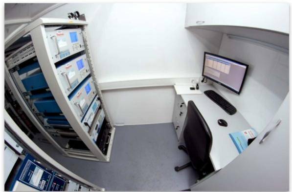
**Measuring car:** the car measures the concentration of PM10 particulate matter, which requires special attention in the autumn-winter period due to adverse meteorological conditions. Moreover, it provides information about pollutant gases in the air and allows samples to be taken for further laboratory tests.
