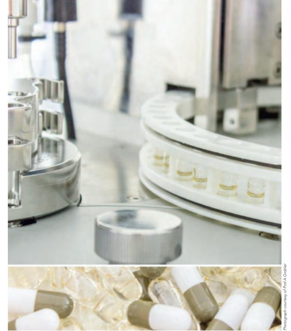
Desktop manufacturing for the novel liquid capsule dosage form of a Pheroid®-containing product now commercially available.
