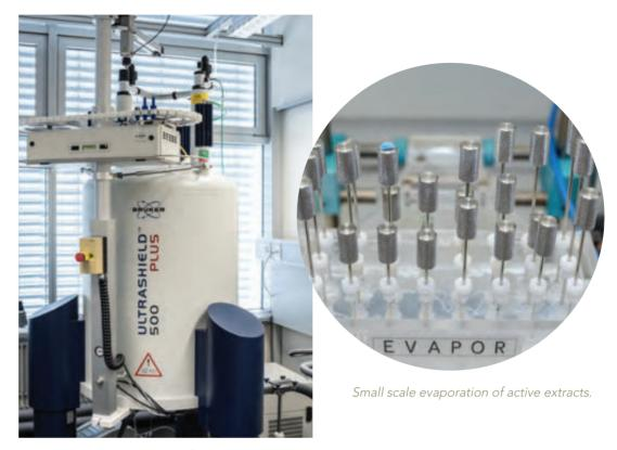
Microprobe NMR instrument for structure analysis.
