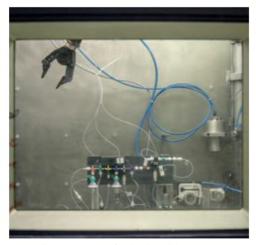
Chemical separation system for Tb radionuclides.
