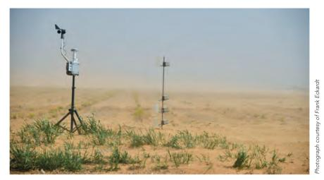
University of Cape Town measuring atmospheric dust concentration and transport in a fallow field, a typical dust source for this region.
