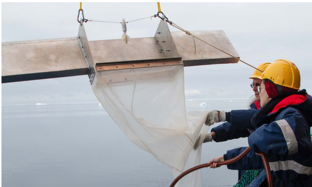
Plankton net used to sample an area of water as part of research into the presence of microplastics in Antarctic waters (Photo: University of Basel, Patricia Holm)
